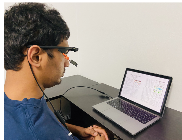
Figure 1: A participant reading the research paper while wearing the Pupillabs Core eye tracker.
