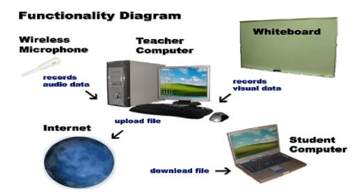
The digital whiteboard will be connected to the classroom PC and all written contents on the board will be captured and converted into vector based graphics. The wireless microphone will capture the instructor's speech and SAVE will synchronize audio and video to produce a single output file. The file can then be distributed to students via the Internet as a download.
