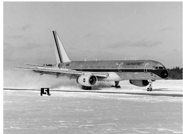
Figure 9: NASA B757 makes a test run on a snowy runway in Michigan.
