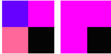
Fig. 7. Correct rendering of PNG (left). IE is unable to properly handle various PNG alpha thresholds (right)
