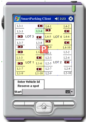
Fig. 4. SmartParking User Interface. A user can view the empty spots and reserve one spot. The reserved spot in this figure is at lot 3 number 4 spot: L3-4
