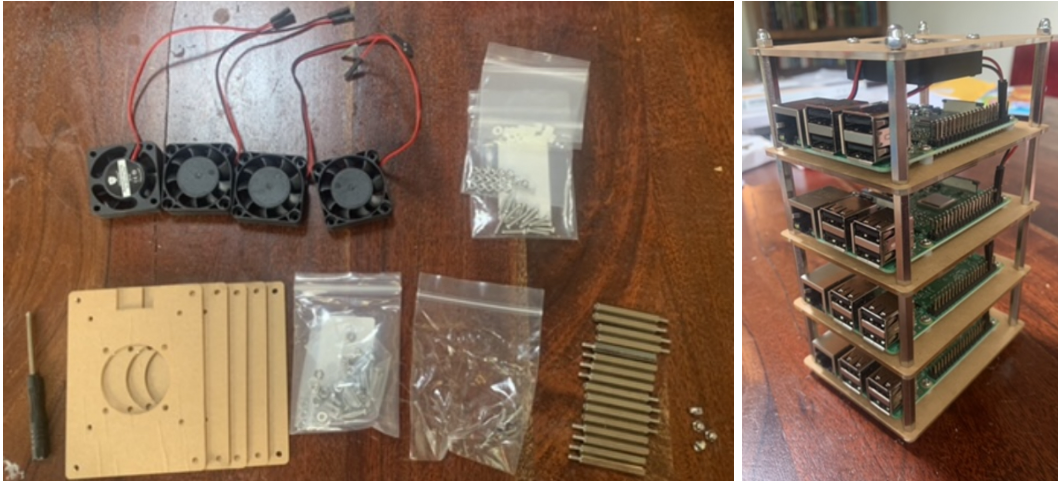
Figure 1: (Left) Components of the Cluster case pre-assembly. (Right) Assembled Cluster.
