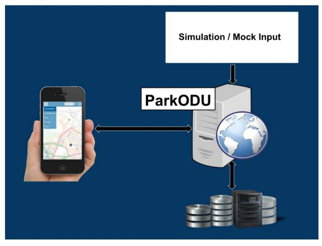
Vehicle detection will be simulated by a REST client application. ParkODU's REST endpoint will receive requests from the vehicle detection simulation's REST client application and update the vehicle counts accordingly. Data from the simulation will be similar to how ODU's parking traffic flows in the real world during a normal weekday and also during special events. The web and mobile applications will process data from the simulation and deliver available parking spaces to the user.
