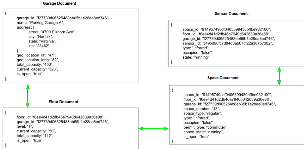
Figure 4: Garage, Floor, Sensor, and Space Document
