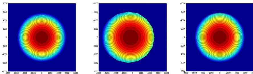
**Fig. 5.** Left: Contours of original, spherical cornea’s height map Center: Contours of cornea model deformed by muscle forces, showing evidence of flattening in the horizontal direction Right: Contours of cornea model deformed by intra-ocular pressure, showing evidence of flattening in the vertical direction, but less pronounced than the flattening caused the muscle forces.
