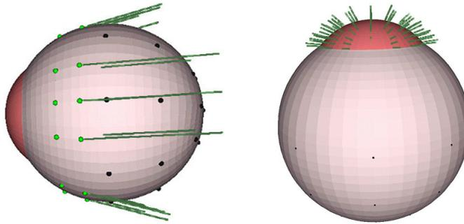
**Fig. 4.** Illustration of two sets of forces applied to the eye. For both sets of boundary conditions, nodes on the posterior portion of the eye remained fixed. These are marked with black dots. Left: Eye model with muscle forces applied tangential to the globe. Right: Eye model with intra-ocular pressure forces applied normal to the cornea.
