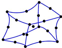
**Fig. 1.** Illustration of the structure of a quadratic hexahedral element. Each edge interpolates 3 nodes, resulting in a quadratic curve. The midpoint of each face and the center of the element also have nodes that support quadratic interpolation across all three spatial dimensions.
