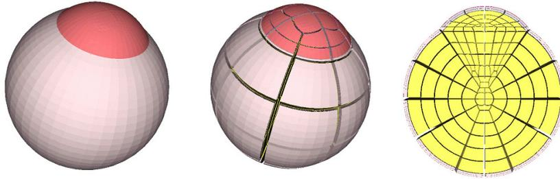
**Fig. 2.** Left: Exterior view of an eye model. Center: View showing divisions between the quadratic hexahedral elements that compose the finite element mesh. Right: Interior view of the structure of the volumetric mesh
