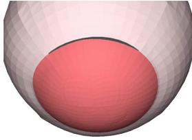
**Fig. 3.** To model an incision along the top edge of the cornea, connections between adjacent elements were removed through all of the corneal layers. Connections between the elements that compose the homogeneous interior of the eye were left intact. The black curve along the top corneal border indicates the placement of the cut.
