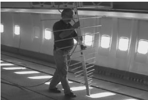
Figure 4. A log-periodic antenna simulating a portable transmitter in the passenger cabin.
