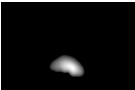
Figure 10. Processed fuel plume image 3 with velocity correction applied
