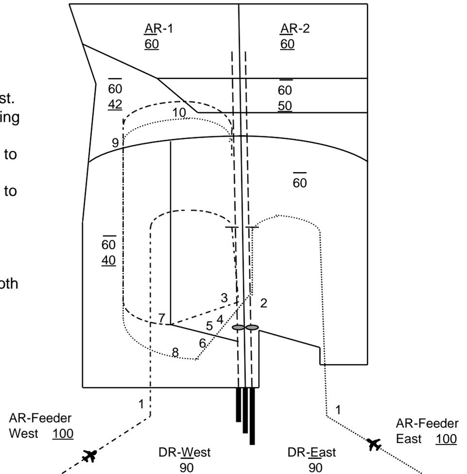
Figure 16. SEA incident scenario 4: RWY 16R straight-in approach; approaches to BFI in progress; EEM right of course.
