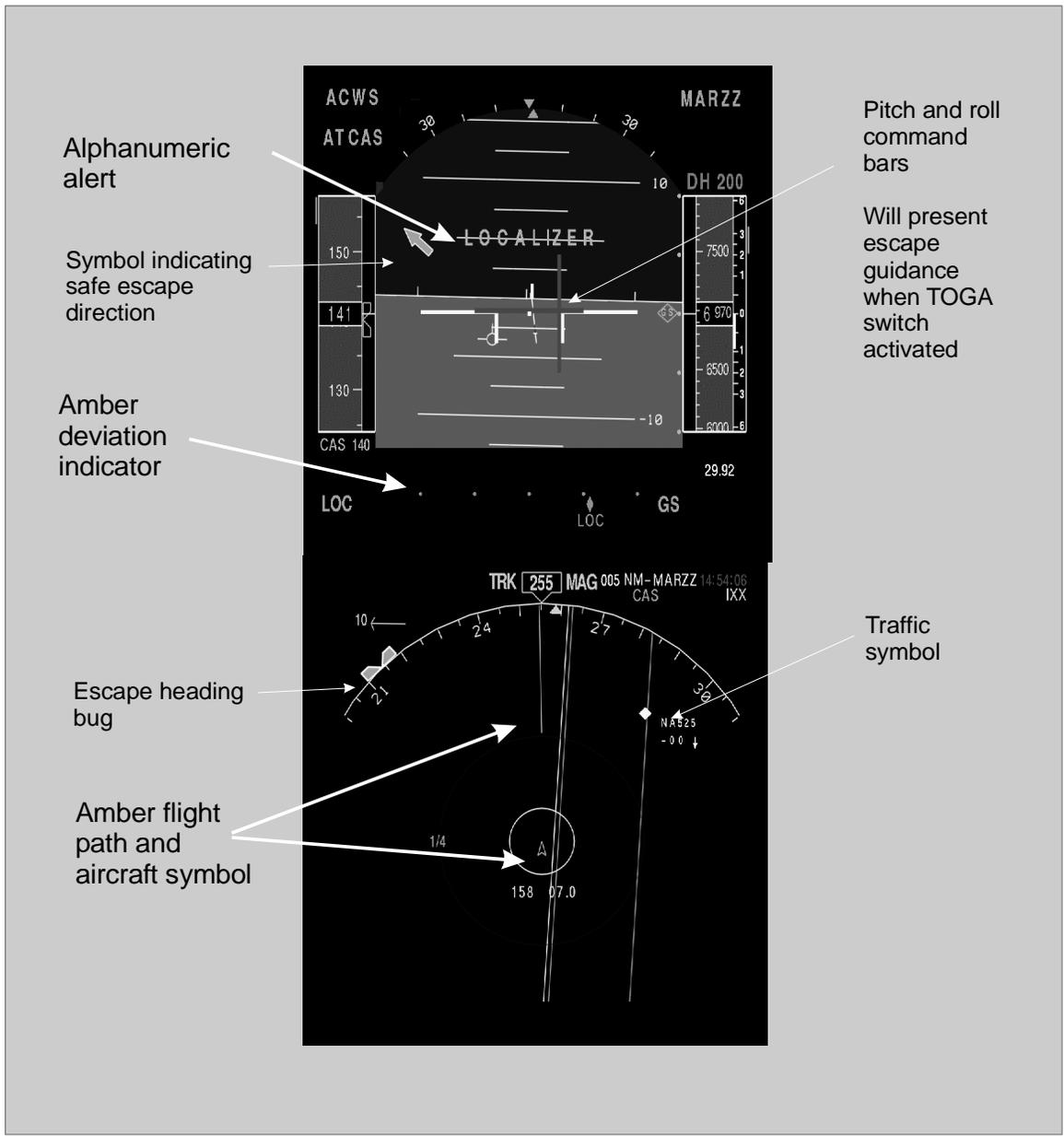
Figure 8. AILS information showing own airplane lateral deviation caution alert (Level two alert uses amber color coding).
