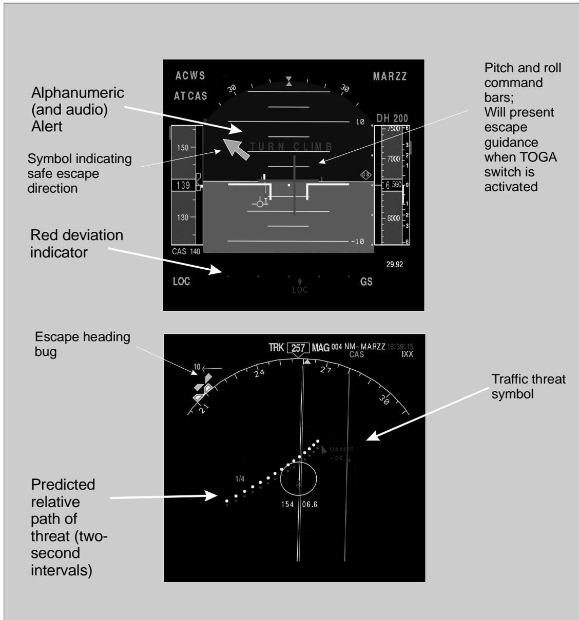
Figure 9. Traffic warning, level three alert (one nautical mile display range, red color coding for level three alert).
