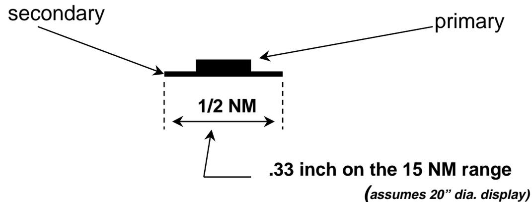
Figure 10. ARTS IIIA/E radar display scaling.
