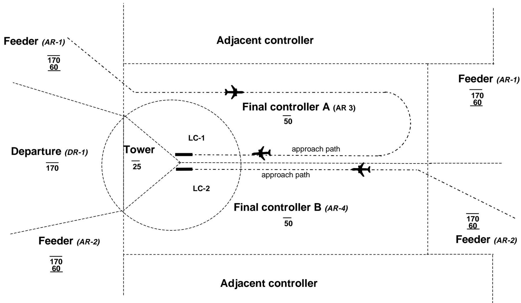
Figure 1. Typical terminal airspace allocation.
