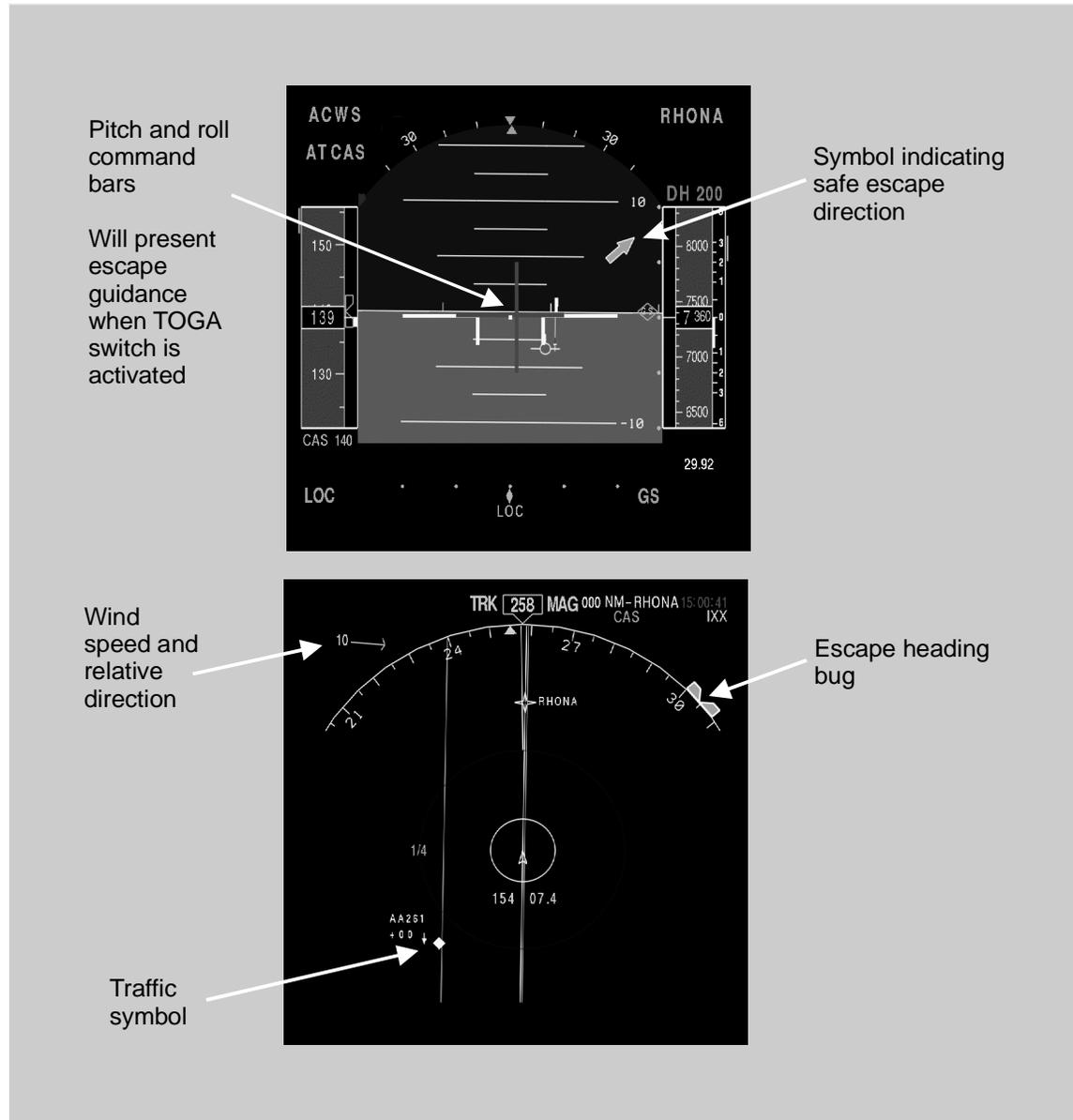
Figure 7. - AILS information presented in the PFD and ND (Nominal condition, no alert, AILS algorithms activated, one nautical mile display range).
