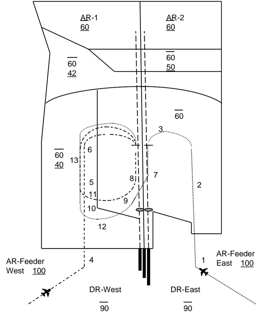
Figure 13. SEA incident scenario 1: RWY 16R straight-in approach, EEM right of course.
