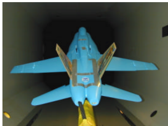
Figure 7. 1/6-scale F/A-18 Model Mounted in the Transonic Dynamics Tunnel
