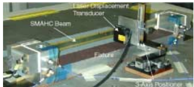
Figure 10: Static thermoelastic experimental configuration.
