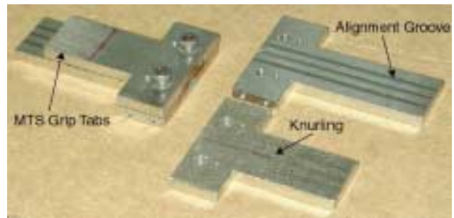
Figure 4: Nitinol gripping apparatus for prestraining and mechanical testing.
