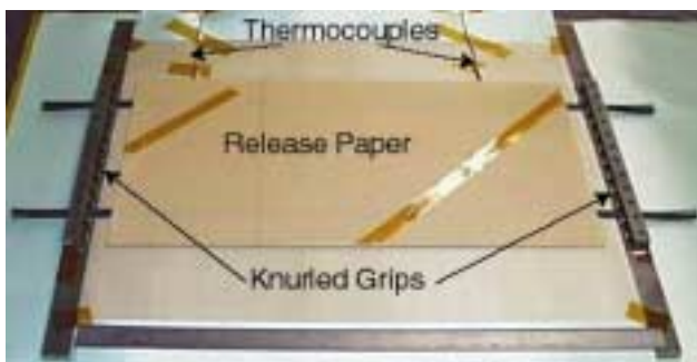
Figure 8: Completed laminate with cure control thermocouples and Nitinol ribbon grips torqued.
