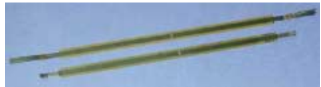
Figure 10: SMAHC beam specimens.
