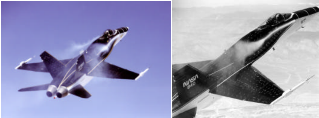
(a) (b) Figure 1. Flow Visualizations of Vortex from the LEX Bursting ahead of the Vertical Tail on an F/A-18 (Photographs Courtesy of the NASA Dryden Flight Research Center)
