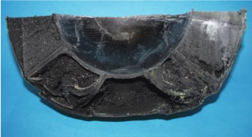
Figure 18 – Photograph of cellular structure cross section, post test.
