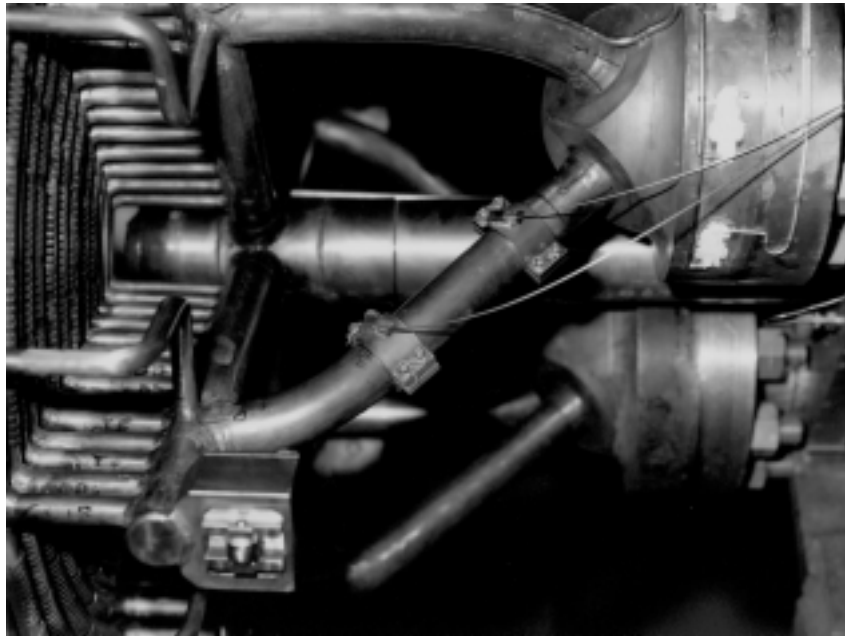
Figure 5. A pair of OFD optical probes integrated onto the 8-ft HTT methane injector
