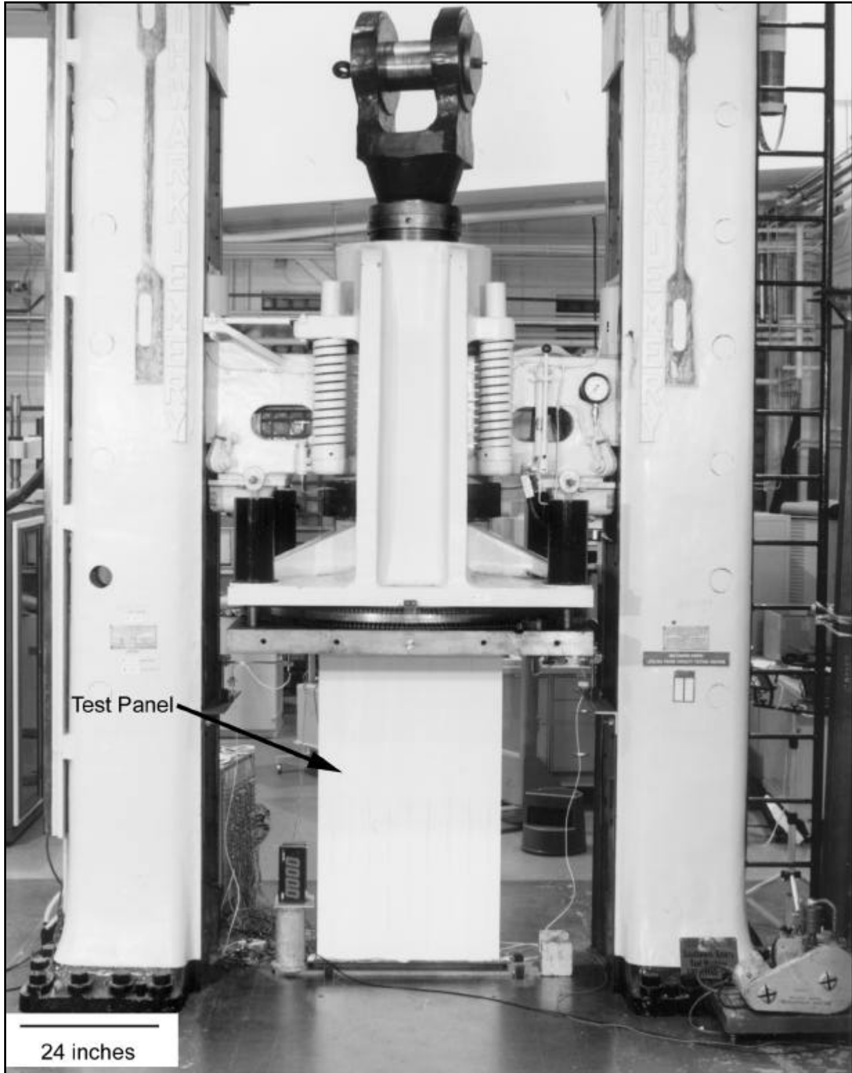
Figure 8. Test panel in the 1000-kip hydraulic test stand.
