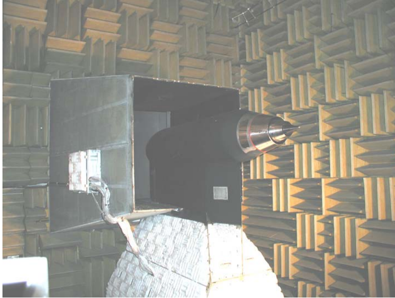
Figure 3. Baseline bypass ratio five separate flow nozzle installed on the jet engine simulator in the test cell of the NASA Langley Low Speed Aeroacoustics Wind Tunnel.
