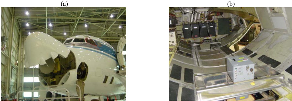
Figure 4. DC-8 equipment - (a) WxR installation, and (b) ALTM installation
