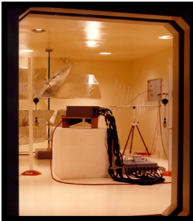
Figure 2. Flight control computer placed in reverberation chamber to collect data.
