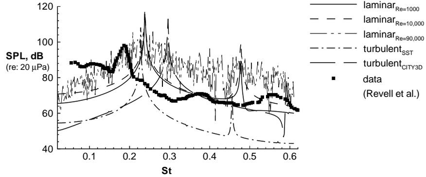
Figure 2. Comparison of predicted and measured sound pressure level for a microphone located  $128D$  away from the cylinder at a  $90$  deg angle to the freestream flow.
