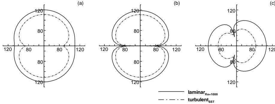
Figure 4. Predicted directivity patterns for  $M = 0.2$  flow traveling left to right. Axes units are decibels (dB, re:  $20\mu\text{Pa}$ ). (a) overall sound pressure level; (b) fundamental frequency; (c) first harmonic.
