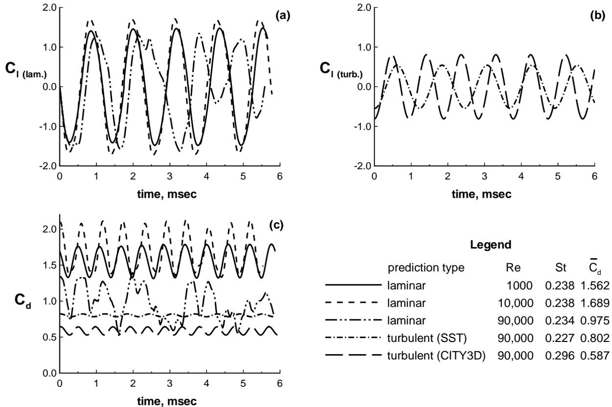
Figure 1. Comparison of predicted  $C_l$  and  $C_d$  time histories for  $M = 0.2$  flow past a 2-D circular cylinder. (a) laminar  $C_l$  predictions; (b) turbulent  $C_l$  predictions; (c)  $C_d$  predictions.
