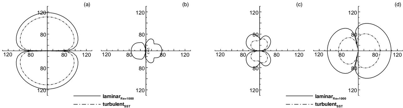
Figure 5. Comparison of the  $C_l$  and  $C_d$  noise components directivity pattern for  $M = 0.2$  flow traveling left to right. Axes units are decibels (dB, re:  $20\mu\text{Pa}$ ). (a)  $C_l$  fundamental frequency; (b)  $C_d$  fundamental frequency; (c)  $C_l$  first harmonic; (d)  $C_d$  first harmonic.
