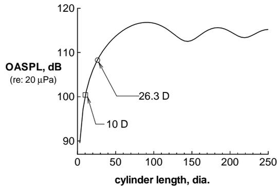
Figure 3. Overall sound pressure level (OASPL) plotted versus cylinder length in the 3-D acoustic computation. The 2-D CFD input data for the turbulent case with the SST model was used for this plot. The CFD data was assumed to be constant along the span for any given source time.
