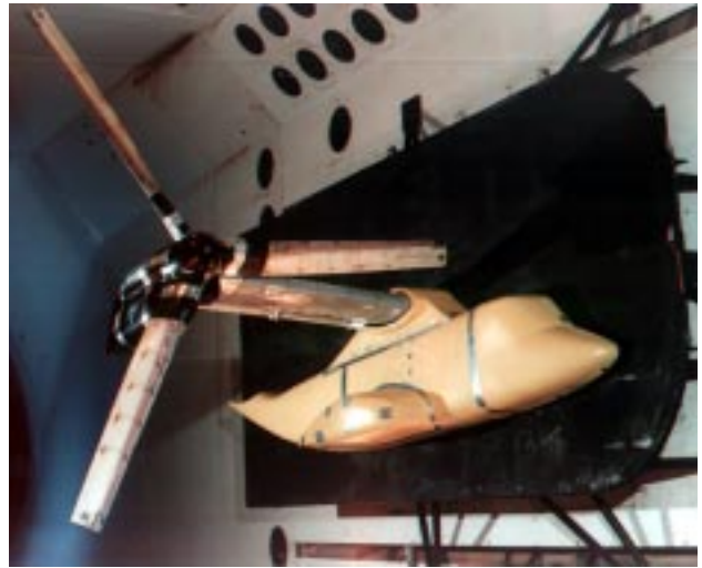
Figure[1]. Model in NASA Transonic Dynamics Tunnel.
