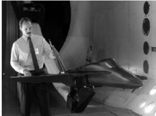
Figure 3. 1/6-Scale F/A-18 Model Mounted in the Transonic Dynamics Tunnel
