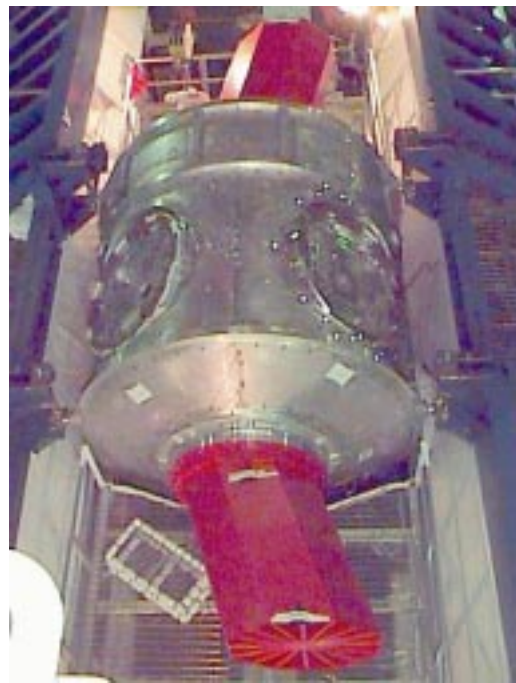
Fig. 2 - Modal Test Configuration
