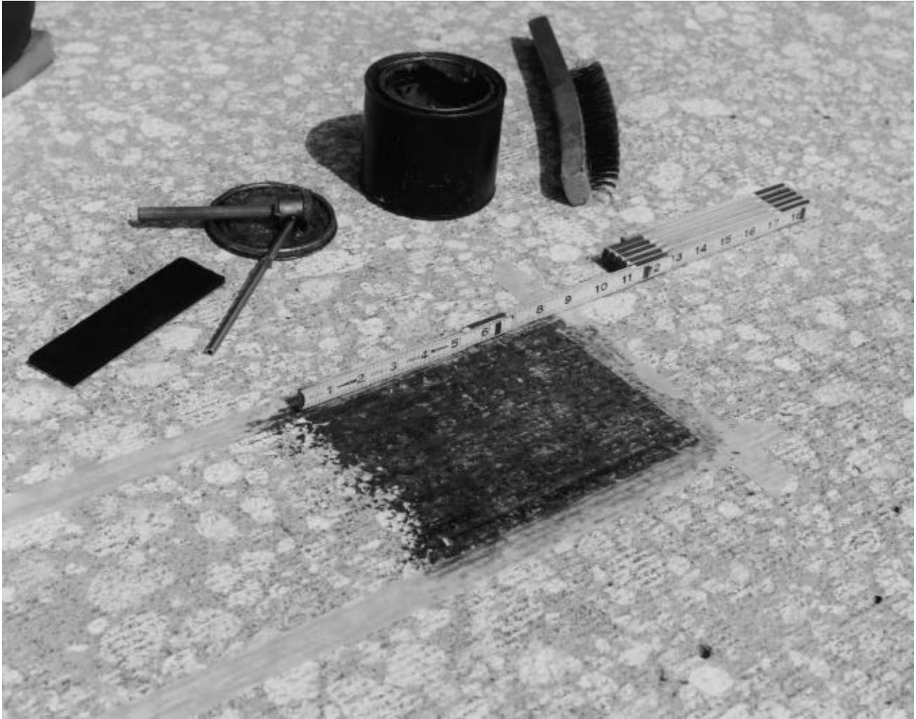
Figure 11. Grease sample texture-measurement kit.
