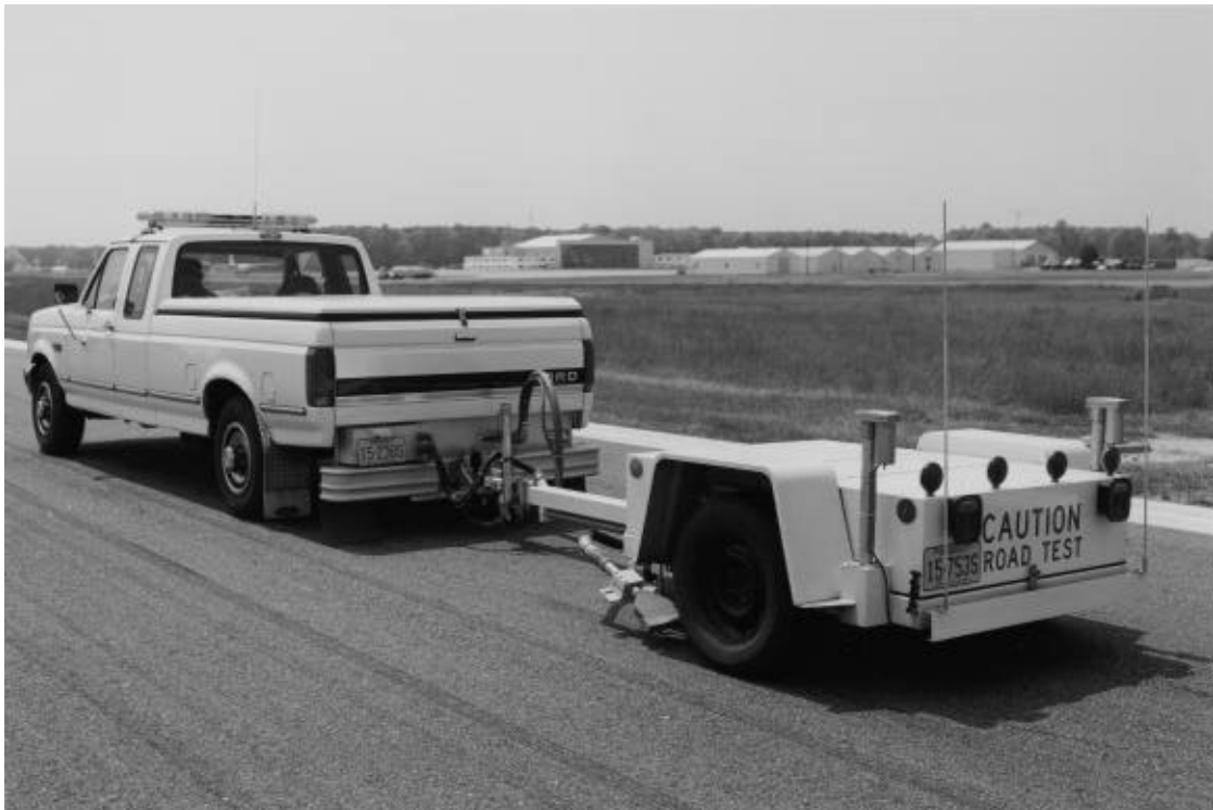
(b) Skid trailer and tow vehicle.
