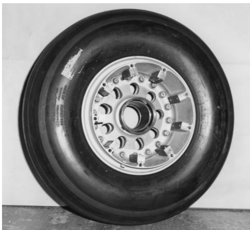
(b) Orbiter main gear tire used during LSRA testing.
