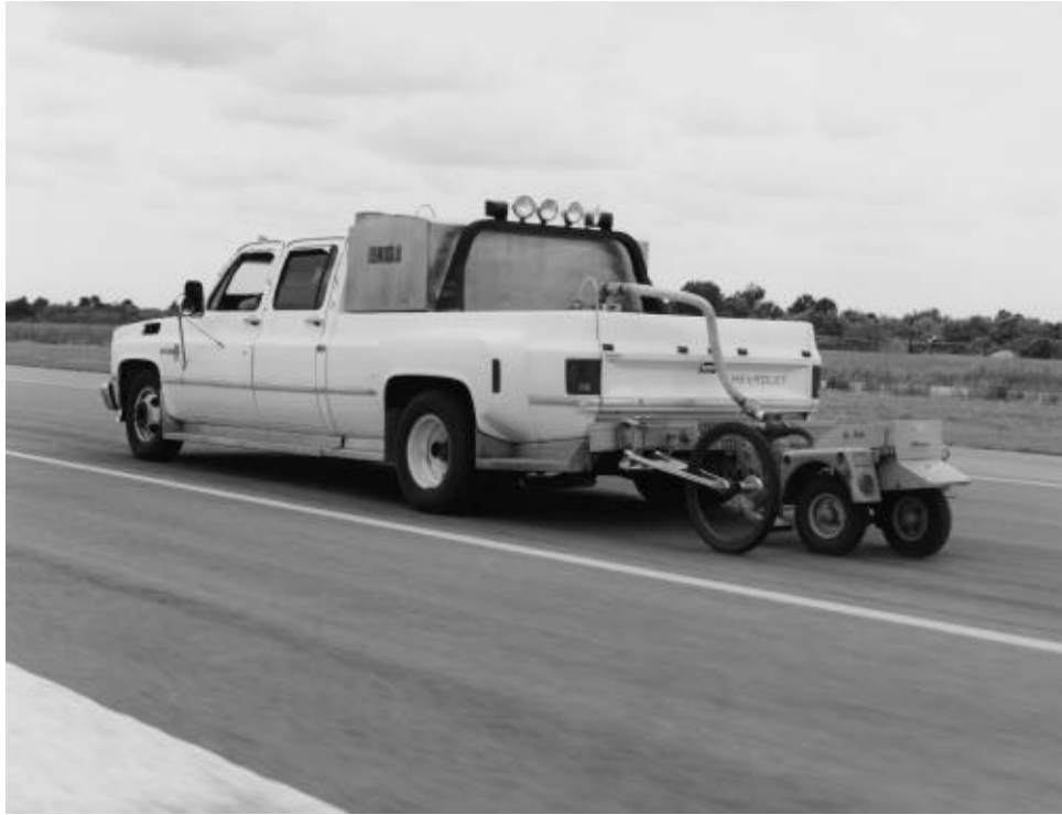
(a) Mu-meter and tow vehicle.
