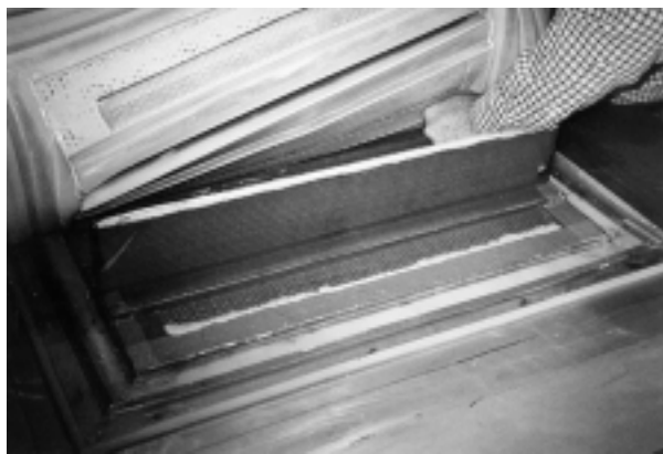
Figure 7. Removal of reusable vacuum bag from VARTM stiffened panel.
