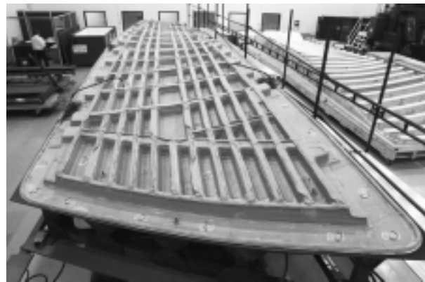
Figure 9. Vacuum bagged semi-span wing tool proof article prior to cure.
