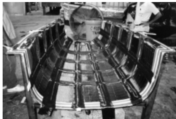
Figure 5a. Vacuum assisted resin transfer molding tooling for fuselage section.
