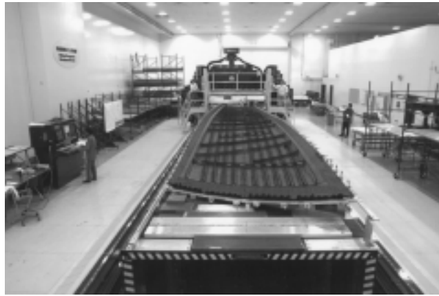
Figure 3. Stitched semi-span wing lower cover preform.
