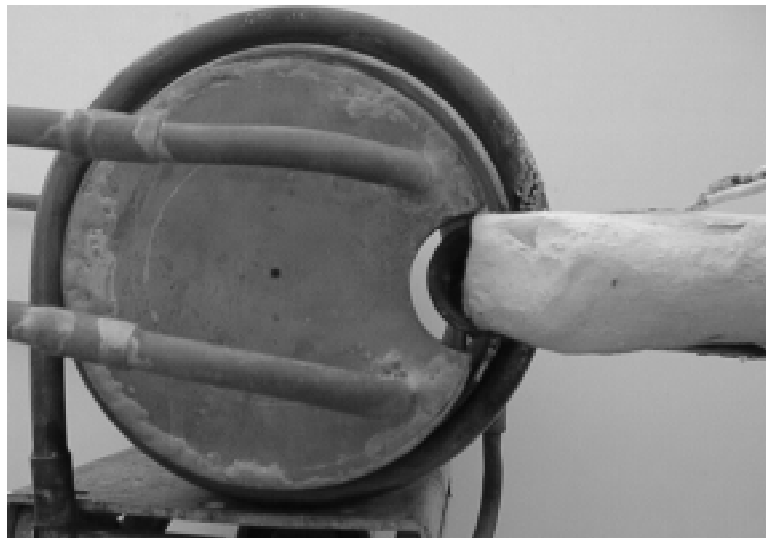
Figure 11: Photograph of insulated heat pipe positioned in rf concentrator.
