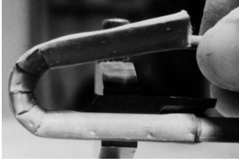
Figure 9: Photograph of the screen wick in the nose region after fabrication.
