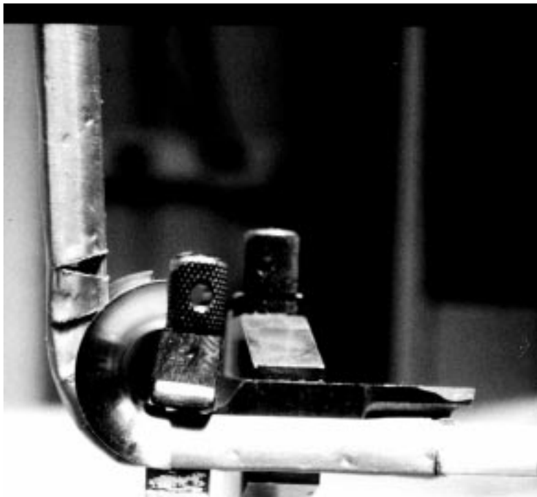
Figure 8: Photograph of the screen wick in the nose region prior to bending around the machined nose part.
