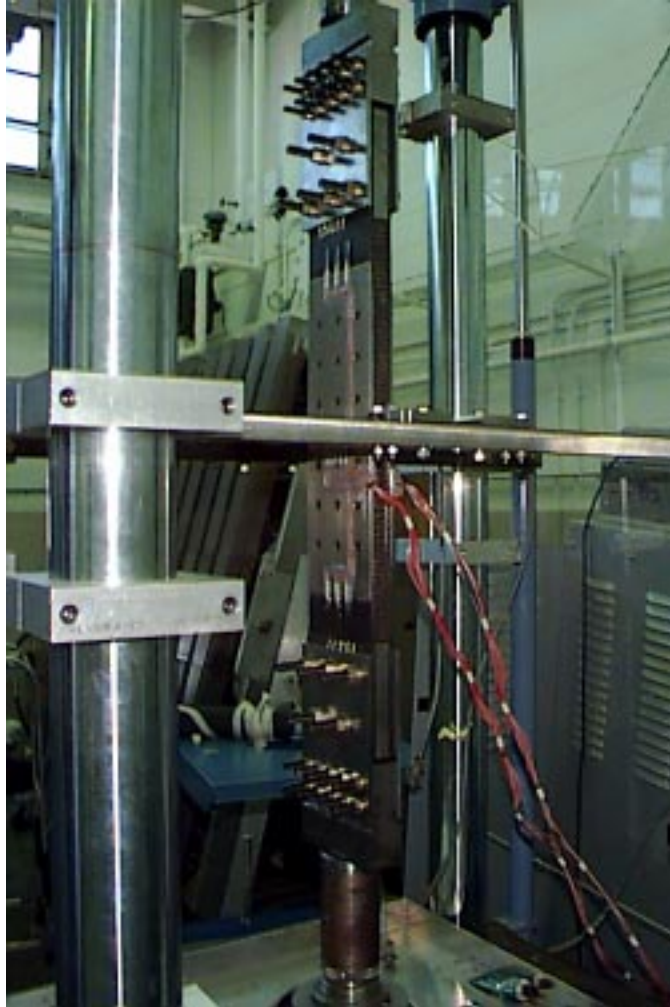
Figure 30. PMC to PMC joint specimen mounted in test machine for fatigue testing.
