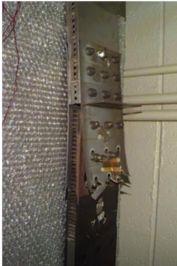
Figure 29. Failed PMC to SPF/DB joint specimen tested at 350°F.
