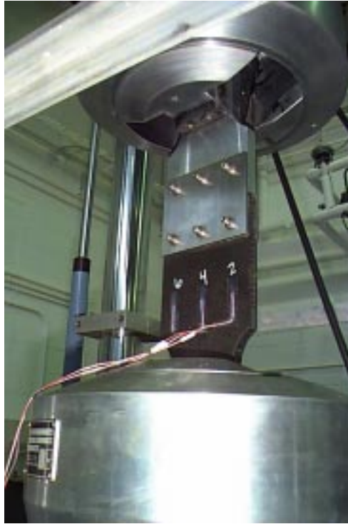
Figure 1. Single-row joint specimen mounted in test machine using hydraulic grips for the room temperature test.
