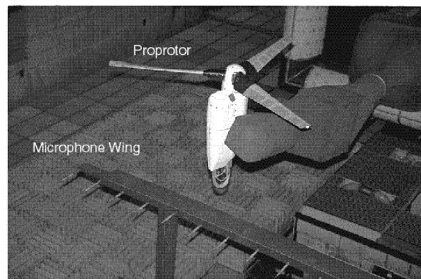
Figure 3. Isolated Rotor TRAM installed in the DNW test section with the microphone wing array located under the rotor.
