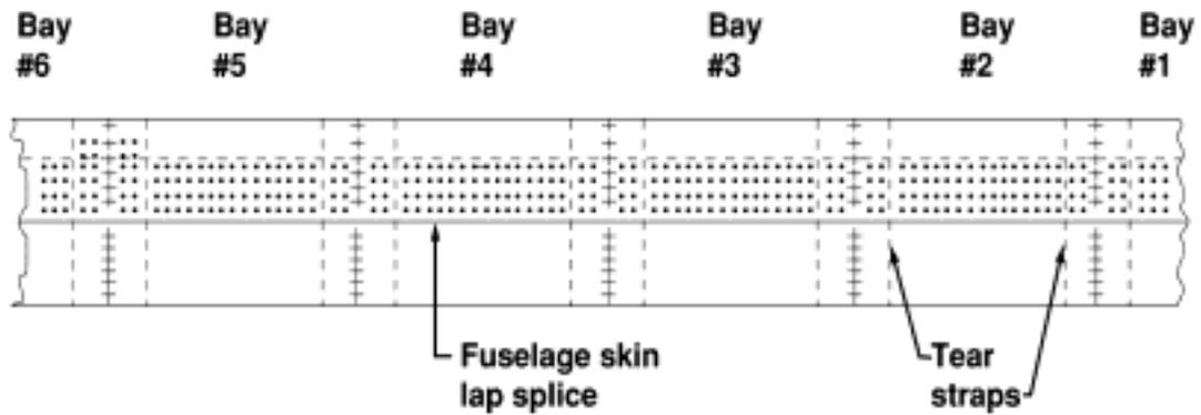
(a) Schematic of fuselage lap-joint panel
