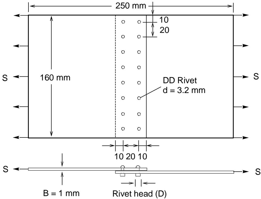
Figure 9. – Riveted lap joint specimen tested by Hartman [27].
