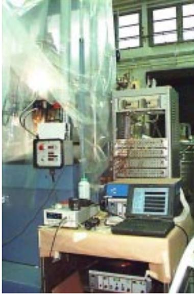
**Figure 8. NDE/IVHM Data Acquisition and Control System.**
