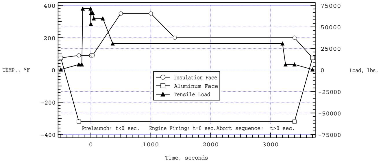
**Figure 12. Flight Simulation Thermal and Mechanical Profiles.**
