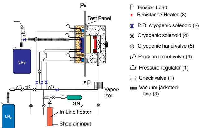
**Figure 9. 1-foot by 2-foot Thermo-mechanical Test Apparatus.**
