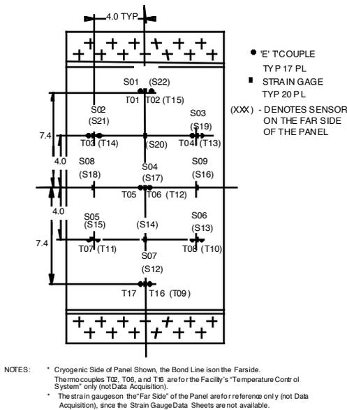
**Figure 5. Instrumentation Layout for the Panel Substrate.**
