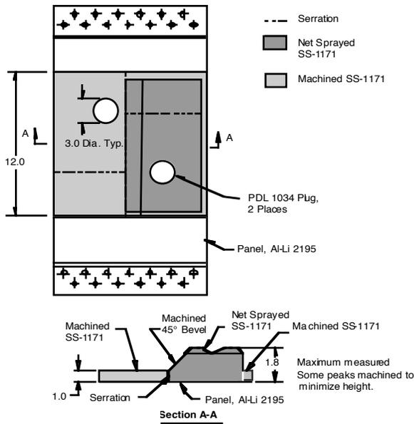
**Figure 4. Cryogenic Insulation Layout.**
