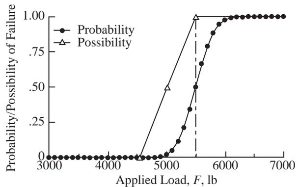
Figure 12. Possibility and probability of material strength failure of the strap.
