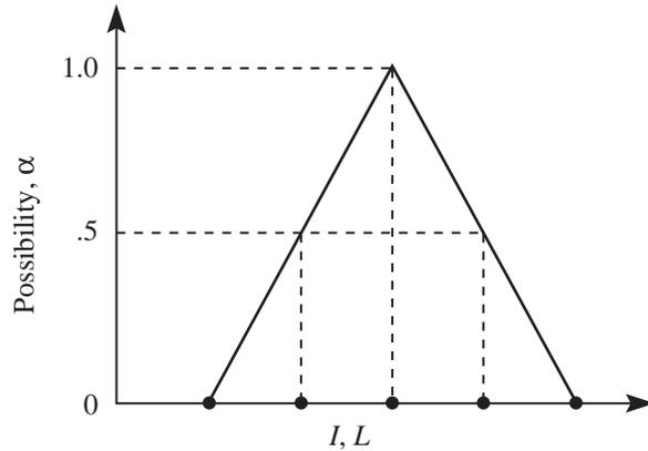
Figure B2. Example membership function for moment of inertia  $I$  and length  $L$  of cantilever beam example. (Filled circles indicate bounds on  $I$  and  $L$  corresponding to  $\alpha = 0.0, 0.5$ , and  $1.0$ .)
