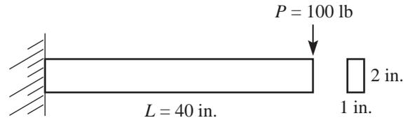
Figure B1. Cantilever beam example.
