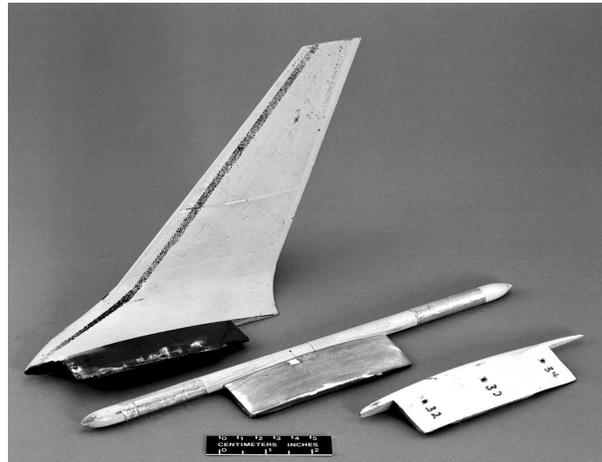
Figure 2 Wingtip configurations: clean wingtip, pencil tipstore, winglet.
