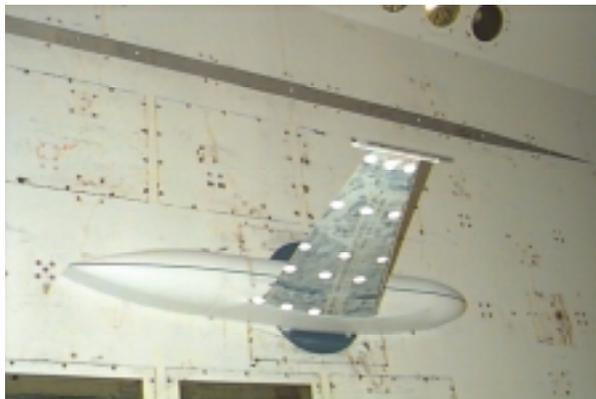
Figure 1 MAVRIC-I model mounted on tunnel sidewall.
