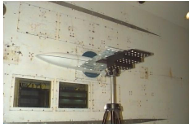
Figure 3 Calibration plate on model wingtip.
