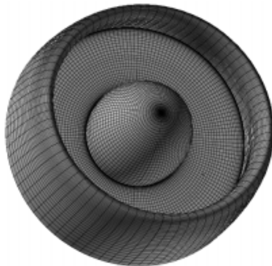
Figure 3. Surface grid for computational analysis of scarf inlet
