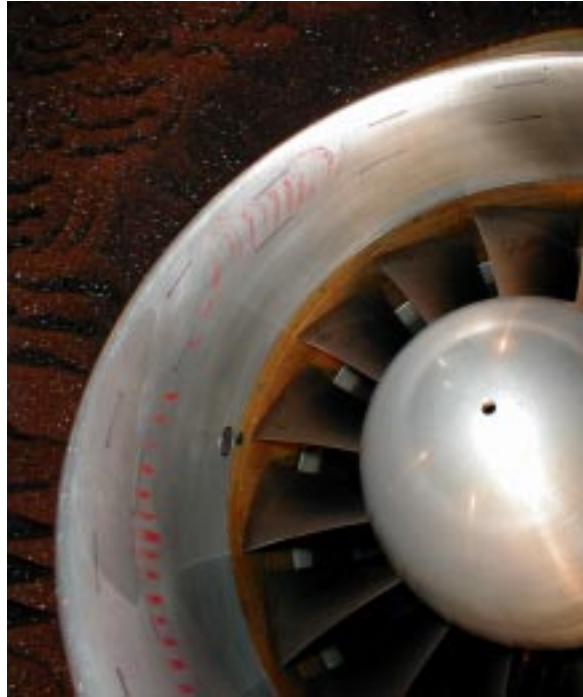
Figure 7. Oil flow test results from run at 90% speed. Location shown is midway between crown and keel
