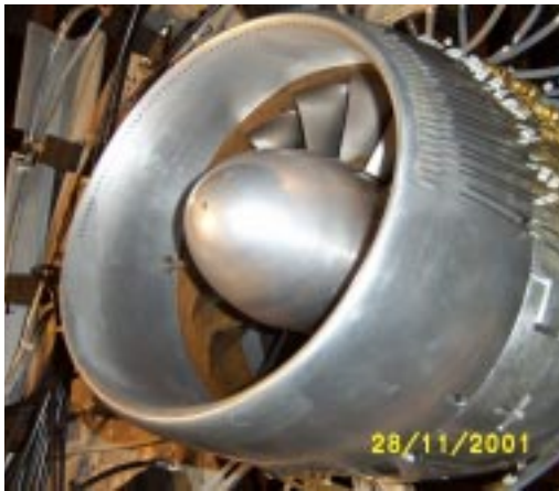
Figure 1. Scarf inlet modified for boundary layer suction over one half of the inlet centered on the crown
