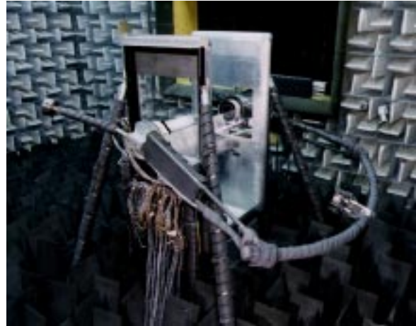
Figure 1. Test apparatus with phased microphone array mounted on pivotal boom in QFF.
