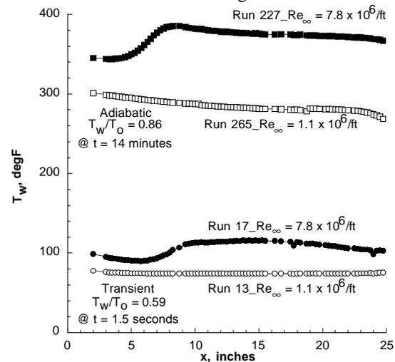
Fig. 5. Comparison of model temperature distributions for recovery temperature (adiabatic wall) and transient heating measurements, 5 deg. straight cone,  $M_{\infty}=6$  (conventional),  $Re_{\infty}=1.1$  and  $7.8 \times 10^6/ft$ ,  $\alpha=0$  deg,  $R_n=0.0001$ -in.
