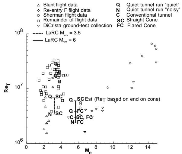
**Fig. 14. Comparison of transition onset Reynolds number on sharp cones near zero angle of attack in flight and ground test as reported in (Ref. 86) with present data.**
