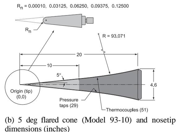
**Fig. 1. Schematic diagram of slender cone models.**
