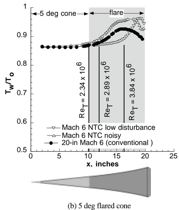
**Fig. 12. Comparison of present smooth body transition onset locations to that obtained in the NASA LaRC M=6 NTC Quiet Tunnel at low and high disturbance levels.  $M_\infty=6$ ,  $Re_\infty=2.8 \times 10^6/\text{ft}$ ,  $\alpha=0$  deg,  $R_n=0.0001\text{-in.}$**
