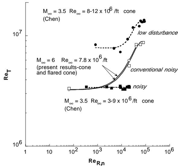
**Fig. 10. Comparison of present nose bluntness effects on smooth body transition to supersonic trends (Ref.10) obtained in the NASA LaRC M=3.5 Quiet Tunnel at low and high disturbance levels.  $\alpha=0$  deg**
