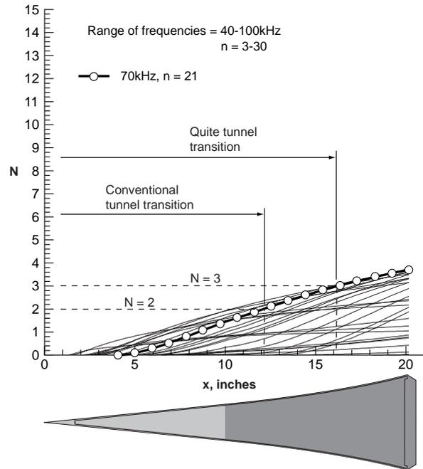
**Fig. 15. Flared cone first-mode N factors of various disturbance frequencies and azimuthal wave numbers  $M_\infty=6$ ,  $Re_\infty=2.8 \times 10^6$ /ft,  $\alpha=0$  deg,  $R_n=0.0001$ -in., adiabatic wall condition**
