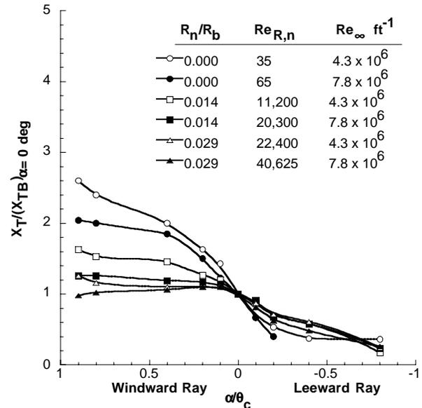
**Fig. 9. Nose bluntness and angle of attack effects on windward/leeward-ray smooth body transition locations. Normalized to blunt cone values, 5 deg. straight cone,  $M_\infty = 6$  (conventional)**
