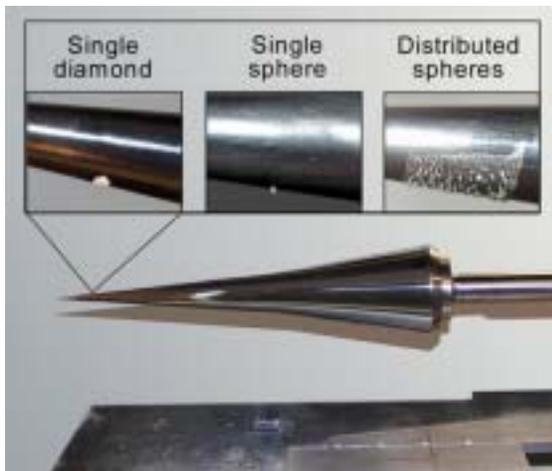
**Fig. 2. 5 deg flared cone (Model 93-10) installed in the NASA LaRC 20-Inch Mach 6 Tunnel (boundary layer trips- inset).**
