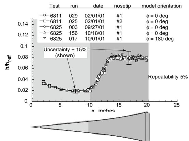
**Fig. 3. Repeatability of heating distribution in conventional Mach 6 Tunnel. 5 deg. flared cone,  $M_\infty=6$  (conventional),  $Re_\infty=4.3 \times 10^6/\text{ft}$ ,  $\alpha=0$  deg,  $R_n=0.0001\text{-in}$ .**
