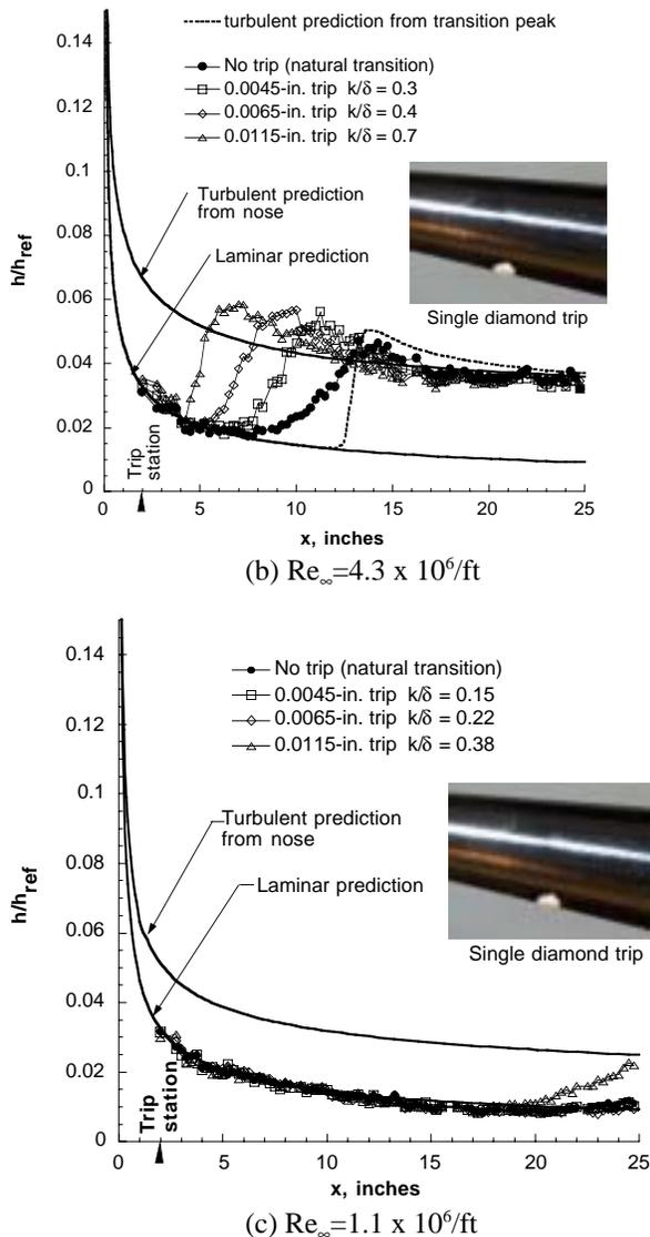
Fig. 4. Comparison of measured smooth and discrete trip heating distributions with laminar and turbulent prediction, 5 deg. straight cone,  $M_{\infty}=6$  (conventional),  $\alpha=0$  deg,  $R_n=0.0001$ -in.
