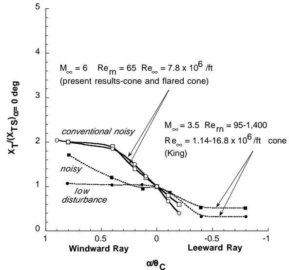
**Fig. 11. Comparison of present angle of attack effects to supersonic windward/leeward-ray smooth body transition locations (Ref. 9) obtained in the NASA LaRC M=3.5 Quiet Tunnel at low and high disturbance levels. Normalized to sharp cone values**
