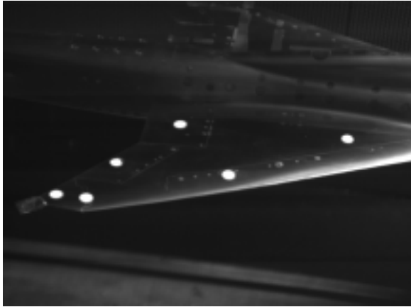
Figure 11. Image of right wing showing polished-paint targets at 3 semispan locations.
