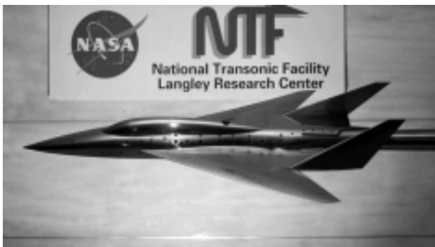
Figure 3. Pathfinder II model with McDonnell Douglas defined wing in the NTF.
