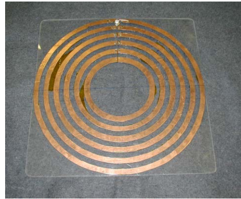
b. Antennae with 0.5 in wide trace of copper foil with various outer diameters
