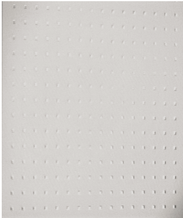
Figure 4. Signal camera image normalized by the reference camera image of the dot target.
