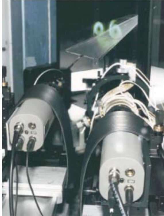
Figure 2. Photograph of the Doppler global velocimeter installed in the Basic Aerodynamics Research Tunnel.
