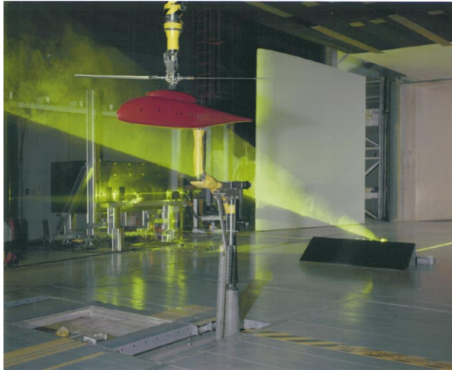
Figure 15. The 1.7-meter isolated rotor system with the fuselage placed below the rotor mounted in the 14-by 22-Foot Subsonic Tunnel.
