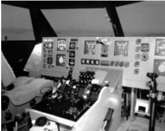
Figure 2. View of VMS cockpit.
