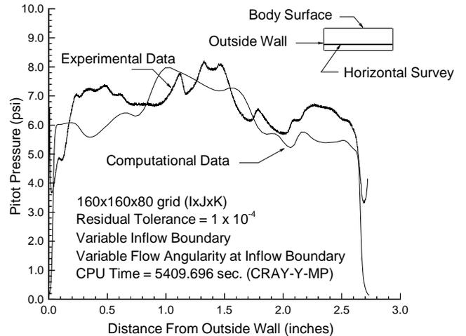
**Figure 10. Computational Exit Plane Pitot Pressure Survey: Three-Dimensional PNS Solution**
