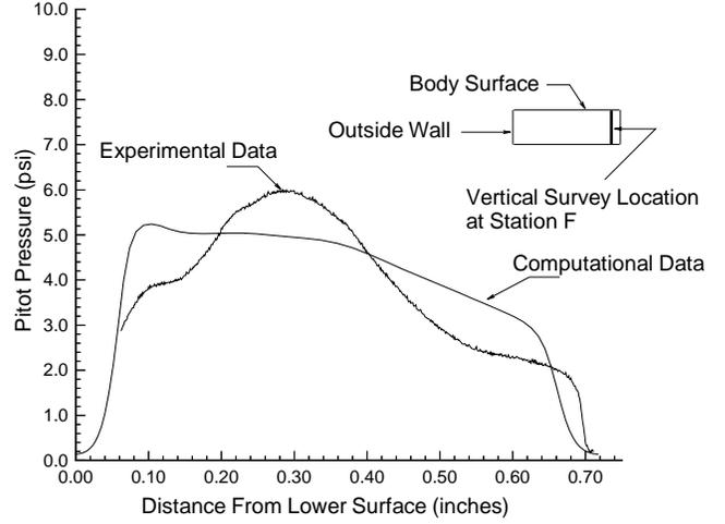
Figure 11(d). Exit Plane Pitot Pressure vertical Survey at Station F
