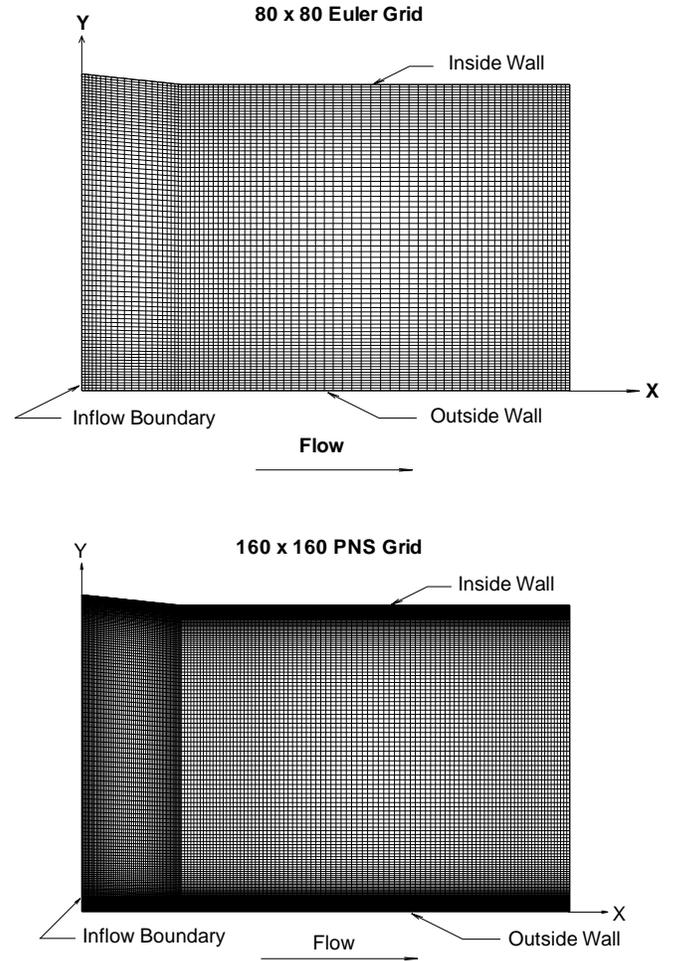
Figure 4. Computational Grids for Two-Dimensional Solutions
