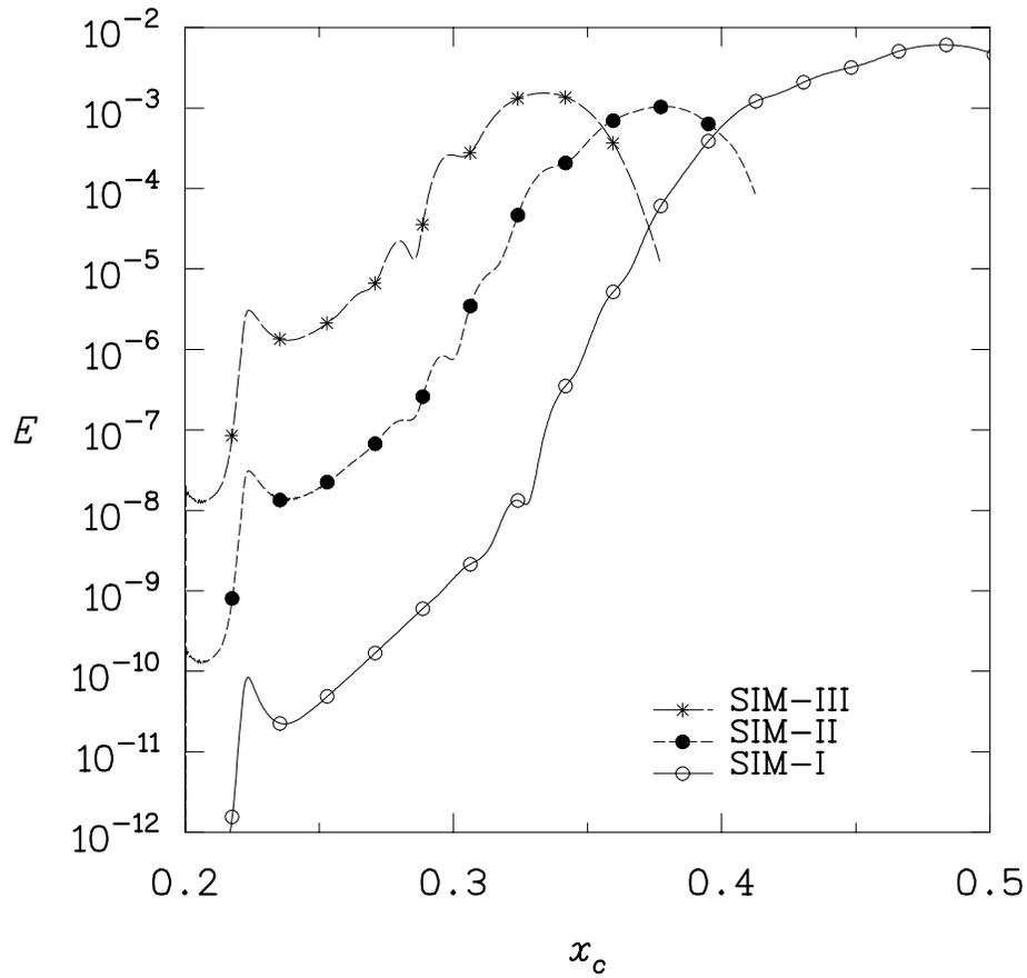
Figure 7. Energy of disturbance velocity with chordwise location for swept-wedge flow.
