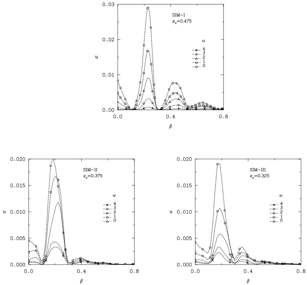
Figure 12. Chordwise velocity decomposed into spanwise wave-number components with frequency at various chordwise locations for swept-wedge flow.
