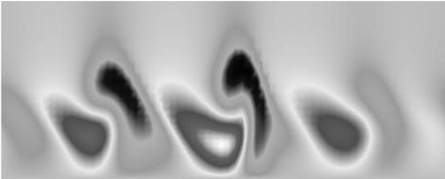
Figure 5. Spanwise planes of disturbance velocity ( $u$ ) contours at chordwise locations for swept-wedge flow of SIM-III.
