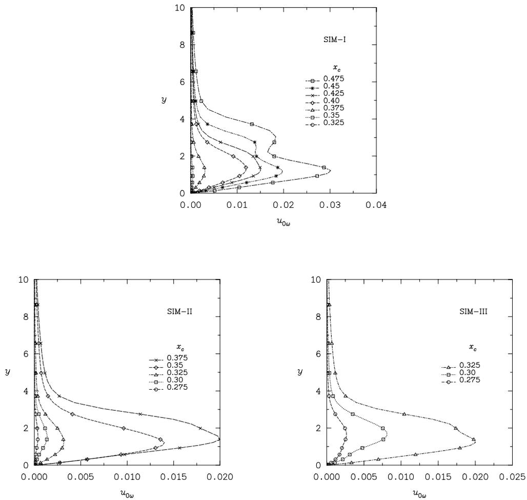
Figure 14. Profiles of crossflow disturbance mode with chordwise distance.
