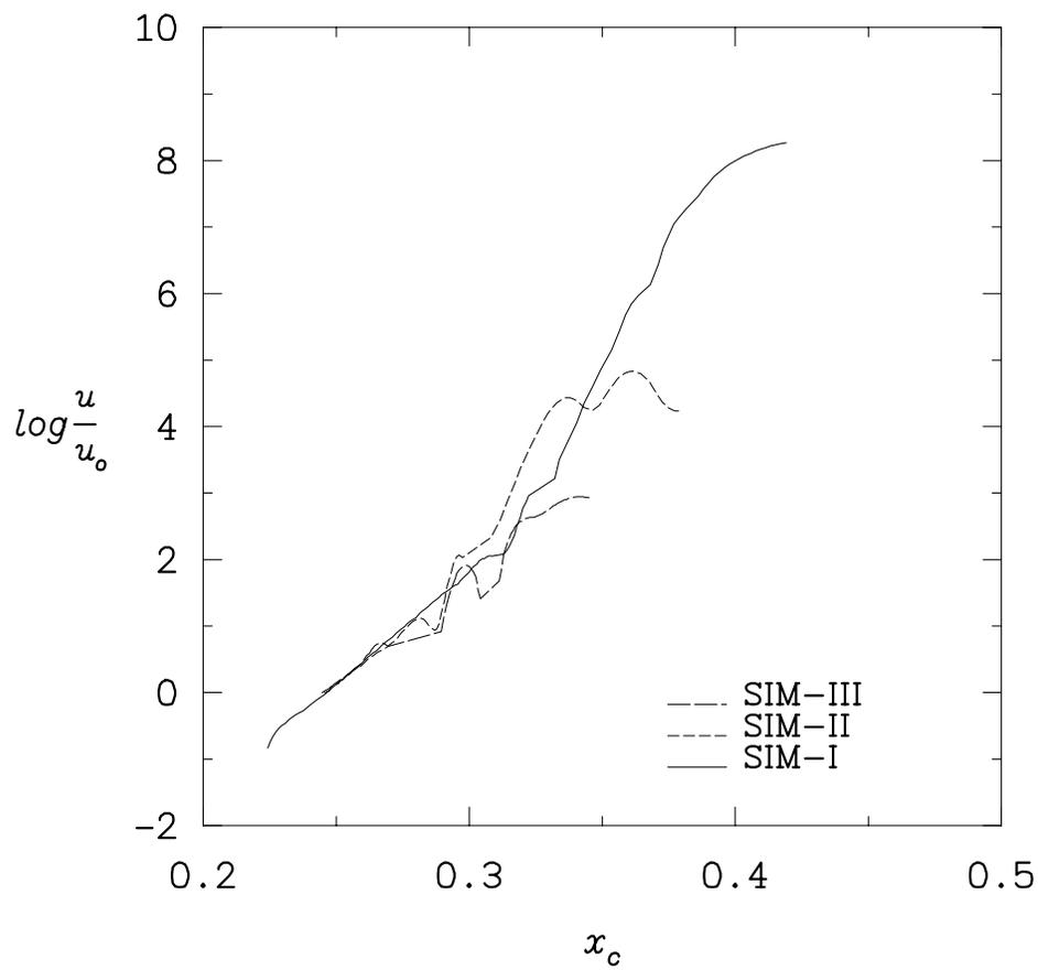
Figure 8. Estimation of  $N$  factor for swept-wedge flow.
