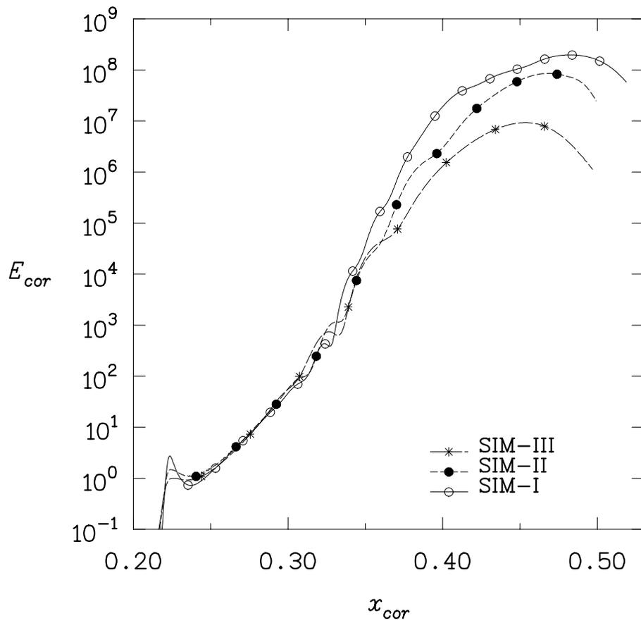
Figure 9. Correlated simulation results for crossflow instabilities in swept-wedge flow.
