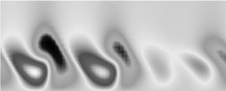
Figure 4. Spanwise planes of disturbance velocity ( $u$ ) contours at chordwise locations for swept-wedge flow of SIM-II.
