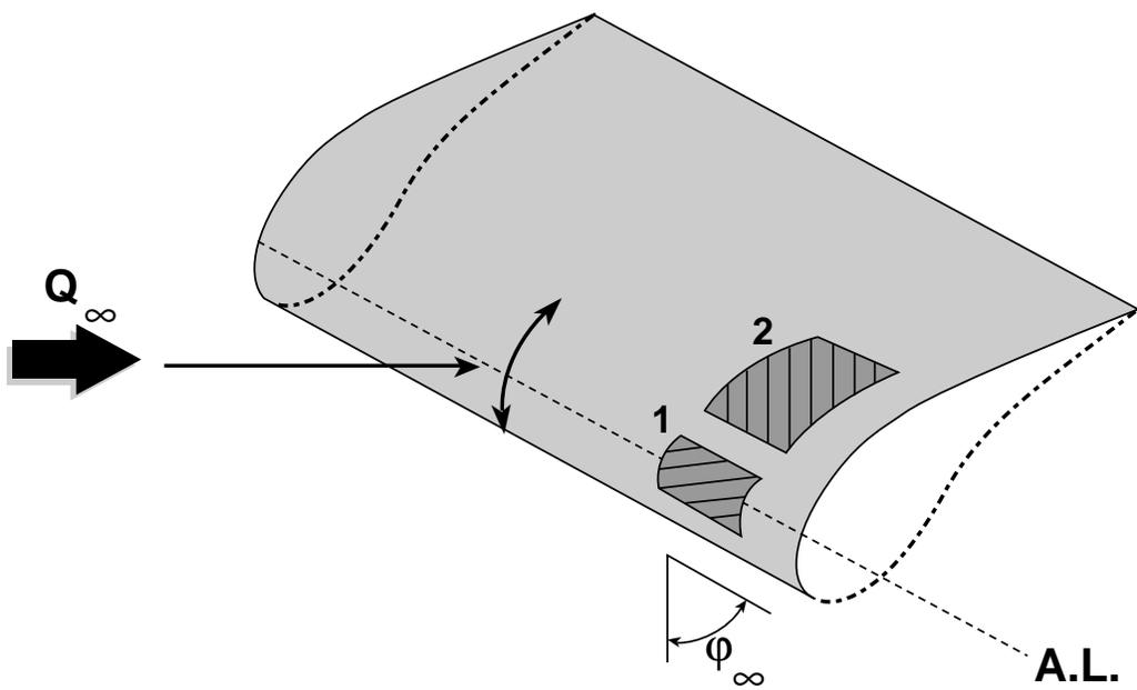
Figure 1. Sketch of swept-wing (1) attachment-line region and (2) laminar-to-turbulent transition region.
