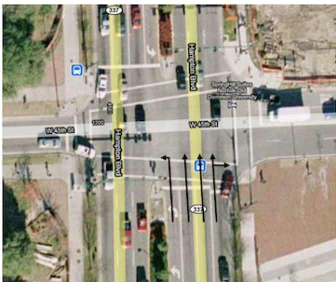
Fig. 3. Intersection of Hampton Blvd. and 45th Street. It shows 4 lanes, 1 is turning left, 2 are going straight and 1 lane is going right/straight.
